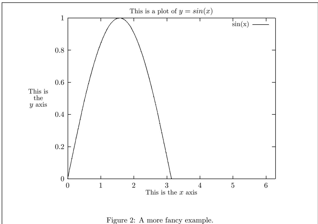
We have requested that the format used by the  $x$ - and  $y$ -axis tic mark labels be in  $\LaTeX$  math mode. This makes the labels look a little better. The default is `set format xy "%g"`. The `%g` represents the general-purpose floating point formatting specification for the `printf` function in C. Any valid floating-point formatting specification, or  $\LaTeX$  command, is allowed in the format.
