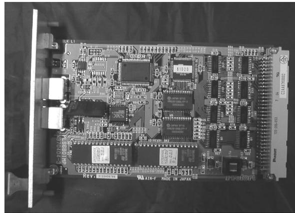
**Figure 1. A Power Supply Interface Controller Module**
